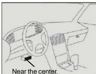
2. Plug the DBScar diagnostic connector into the vehicle's DLC. It is suggested to use the OBD II extension cable to connect the DLC and the DBScar connector;
